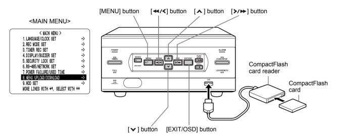
You can save menu setting values onto a CompactFlash card. This sub-menu also lets you read menu setting values saved on CompactFlash cards.
